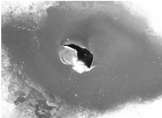
FIGURE 9: Burned Through Heat Exchanger
